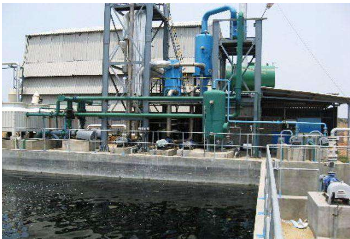
Fig. 10 Mechanical Evaporator Ancillary Unit
