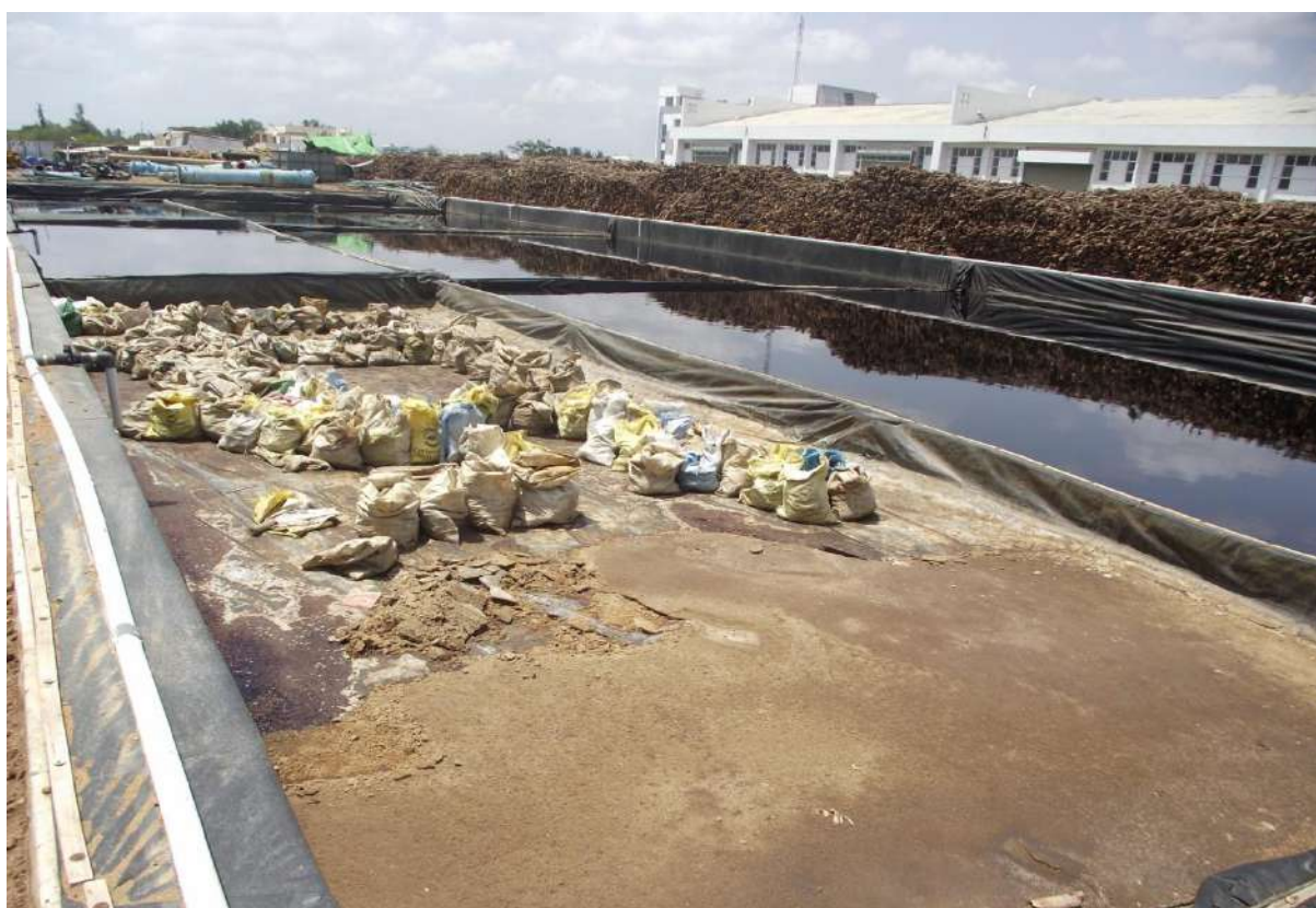
Fig. 14 Mixed salt collected from Solar Evaporation pan
