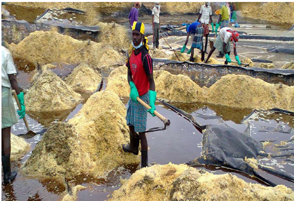
Fig. 15 Mixed salt collected from Solar Evaporation pan
