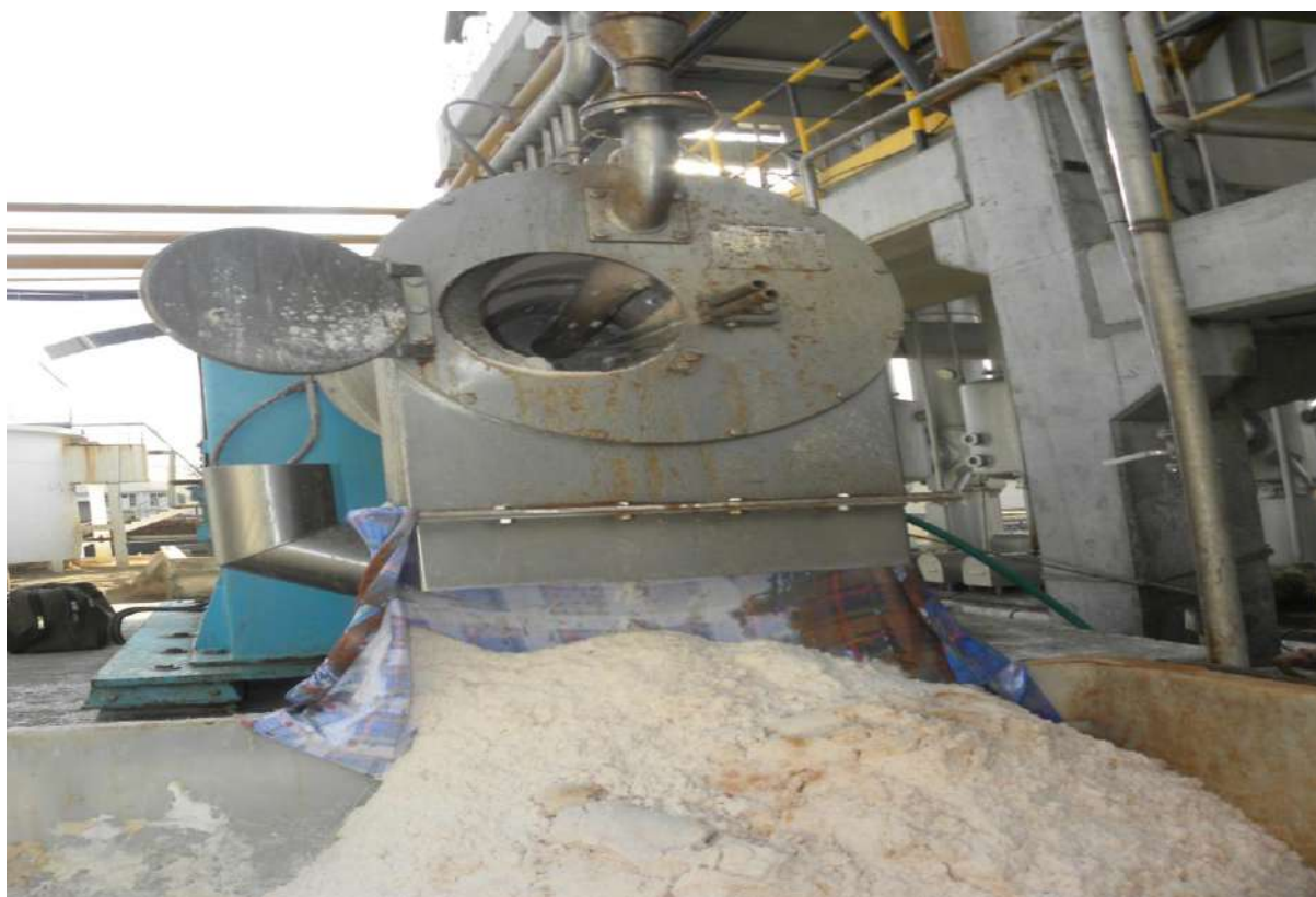
Fig. 13 Salt collected from Crystallizer
