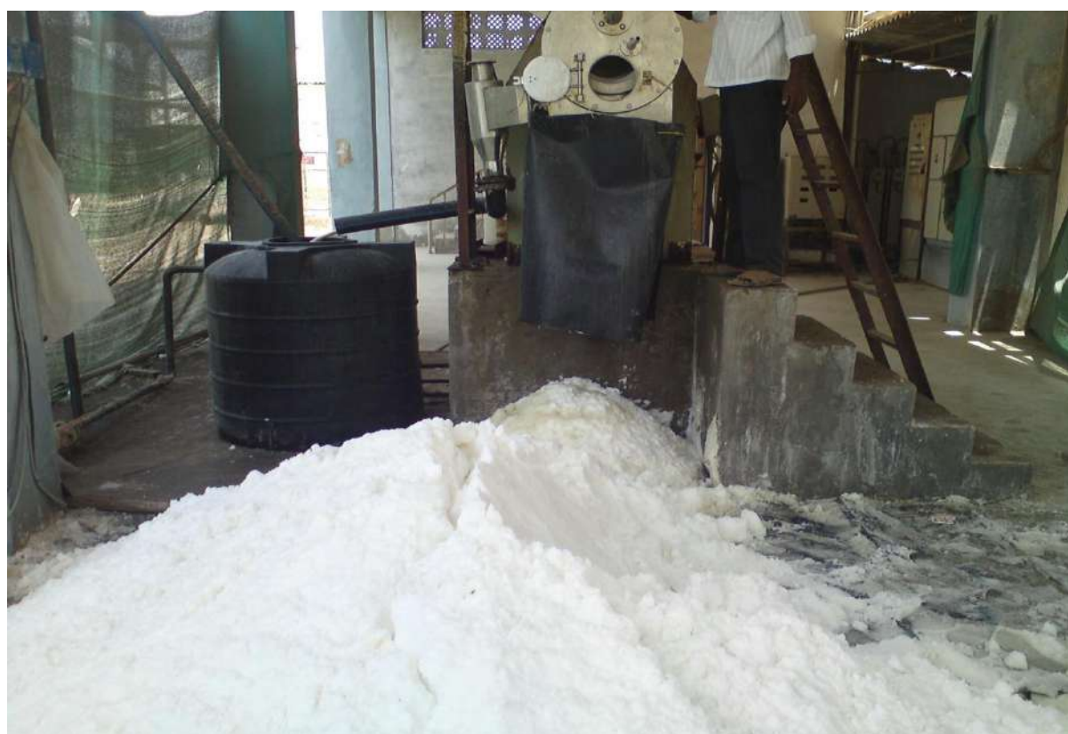
Fig. 12 Salt collected from Crystallizer
