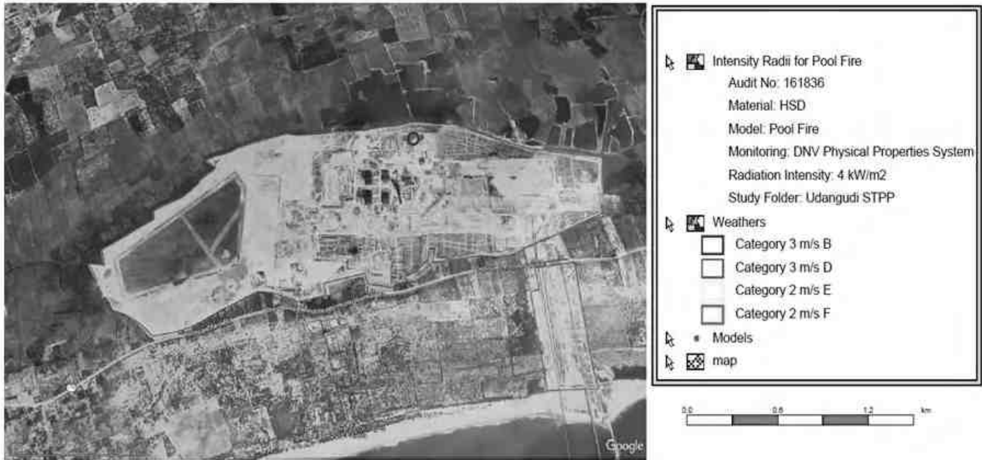
Figure 7-3 Thermal Radiation Radii for late Pool Fire Due to Rupture of HSD Tank
