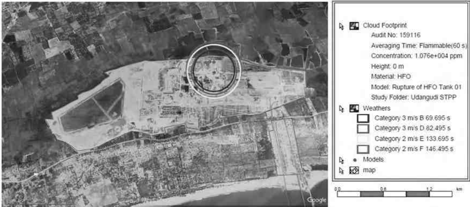
Figure 7-2 Flash Fire Envelope Concentration of HFO Vapours due to Rupture of HFO Tank
