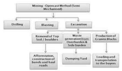
**Figure 2-15 Schematic Diagram of Mining Process**
