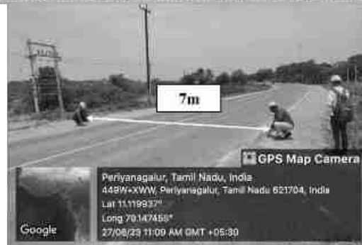
Measurement of SH-139 road width of 7m in the south side
