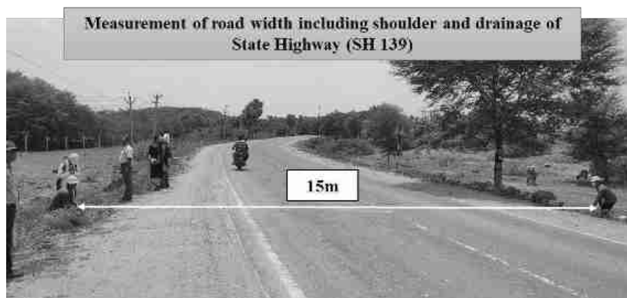
Figure 4. Measurement of road width including shoulder and drainage of SH 139 road
