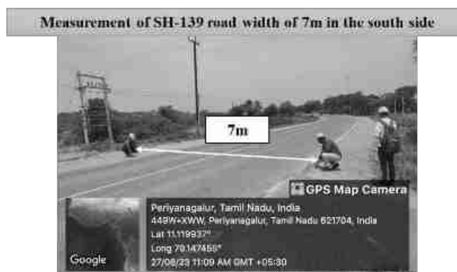
Figure 3. Measurement of SH-139 road width of 7m in the south side
