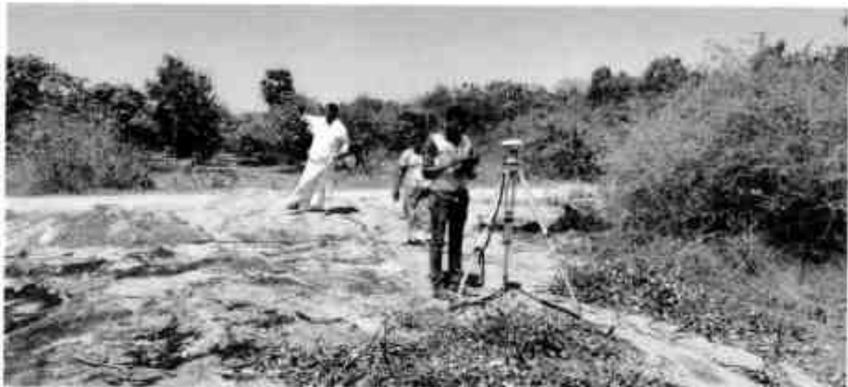
Fig.1 Photographs showing DGPS Survey of the Base Point
