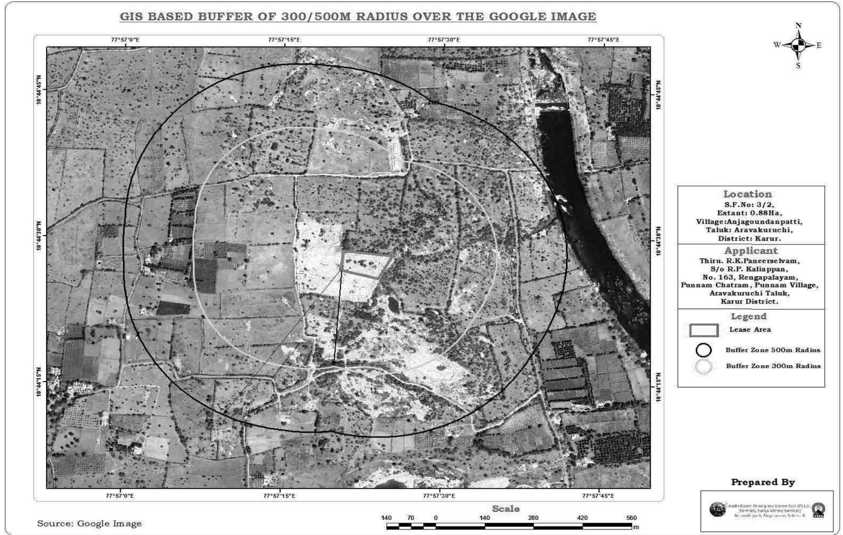
Fig No. 1.3: Google Earth Image showing 300m and 500m radius around the proposed Ordinary stone and gravel quarry
