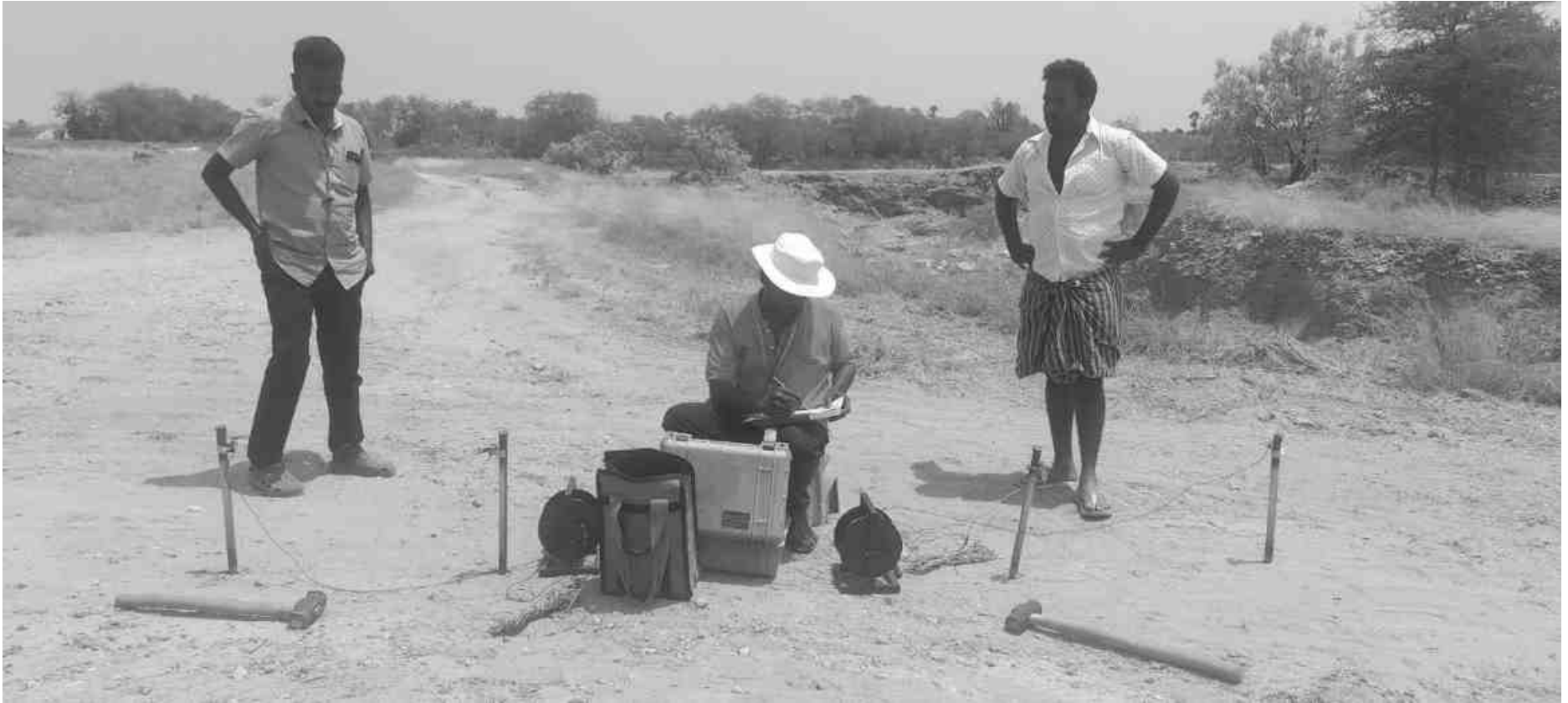
Figure 7 Photograph showing the Geophysical survey on the project Location
