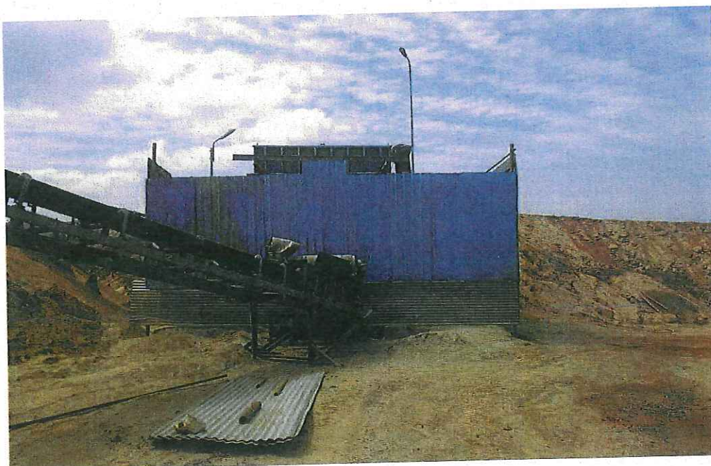
Primary Crusher- MS cover with water Spraying Arrangement
