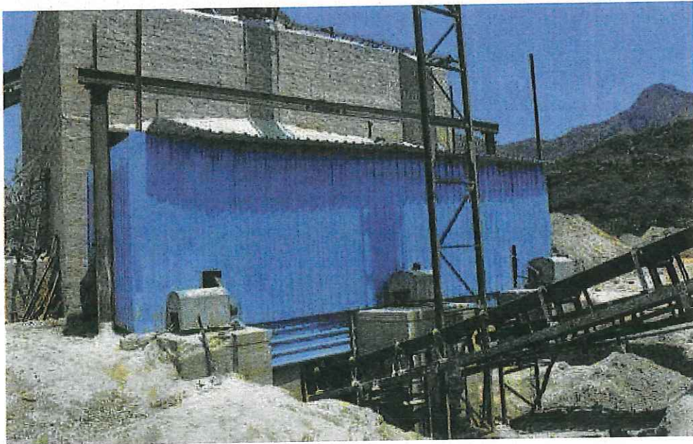
Secondary Crusher - 3 Nos - Common MS cover with water Spraying Arrangement
