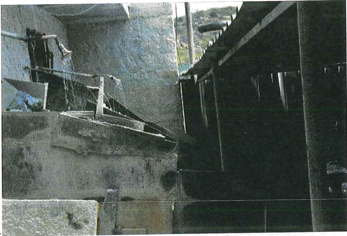
Secondary Crusher - 3 Nos - Common MS cover with water Spraying Arrangement
