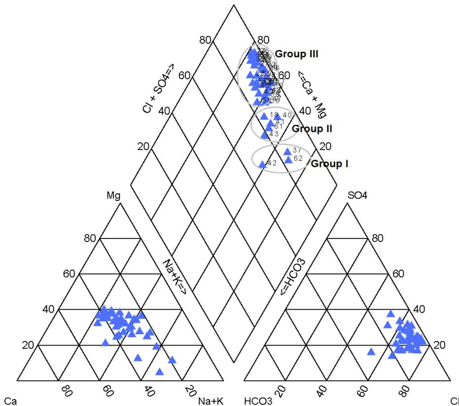
Fig. 9: Piper plot of groundwater samples.
