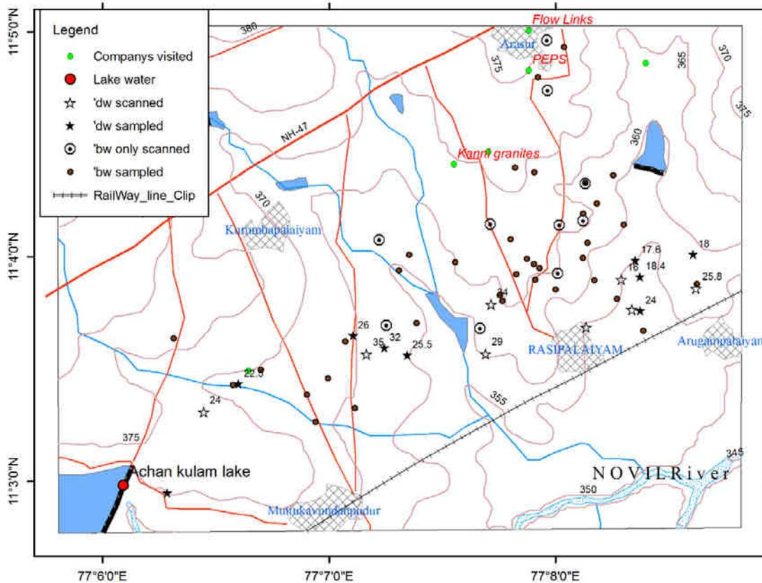
Fig. 3: Groundwater levels (approximate) measured in the dug wells during the field work (many wells pumps are in running condition).
