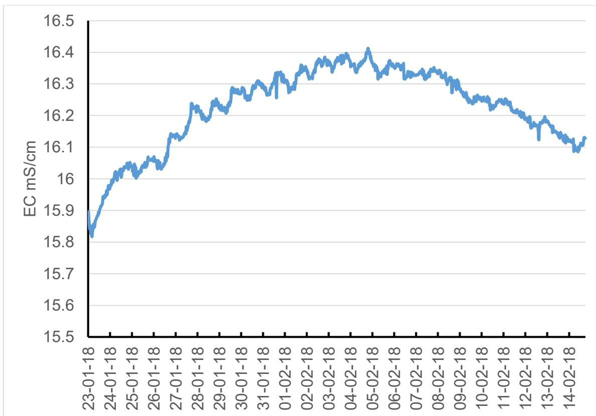
Fig. 10: Electrical conductivity of groundwater monitored in real time at 30-minute interval in the dug well of Mr. A. K. Jaganathan.
