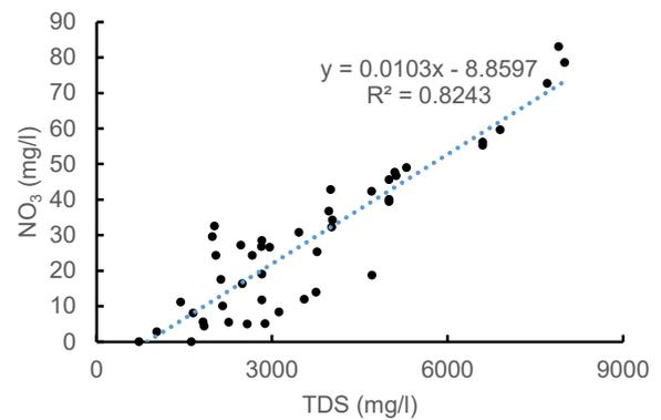
Fig. 8: Plots showing total dissolved solids (TDS) vs different ion concentrations in groundwater
