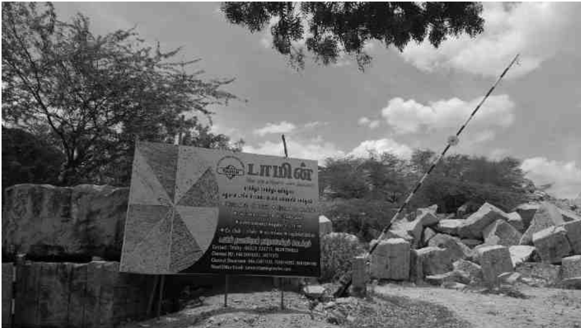
Tvl.TAMIN Ltd. Naganur village , Kulithalai Taluk latitude 10° 44' 30.27" Longitude 78° 23' 53.03" ,Multicolour Granite. N30°W, 70°Southerly dipping.
