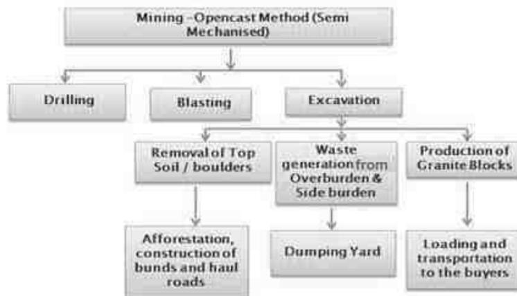
**Figure 2-15 Schematic Diagram of Mining Process**
