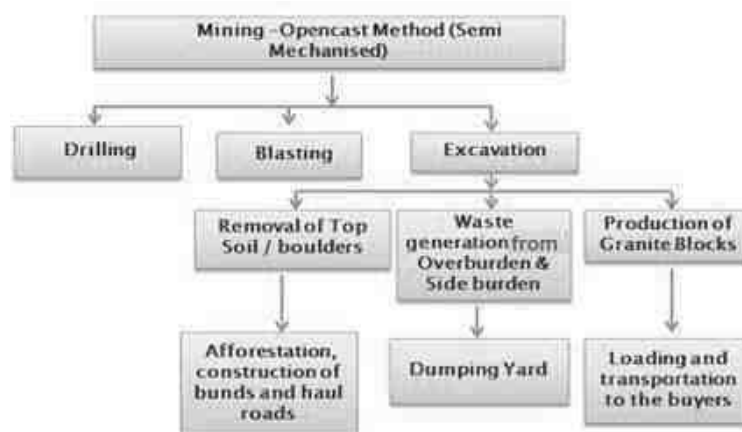
Figure 2-15 Schematic Diagram of Mining Process
