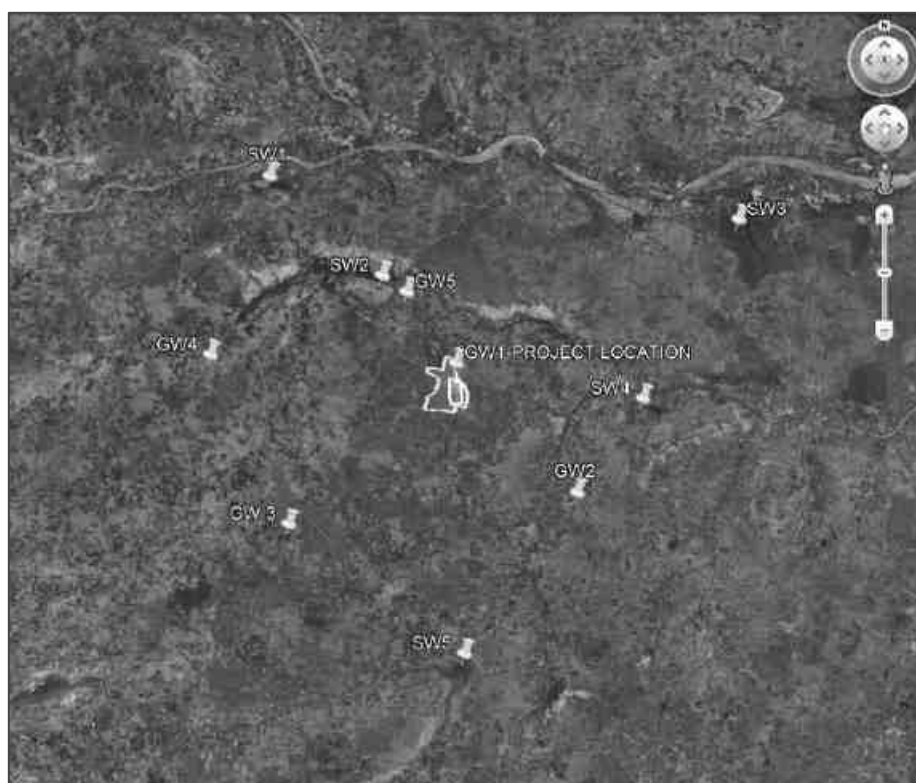
Figure 3.16: Surface and Groundwater Quality Monitoring Locations
