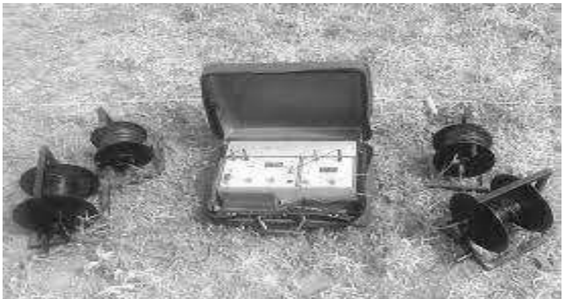
Figure 3.11. DDR-3 Electrical Resistivity Meter
