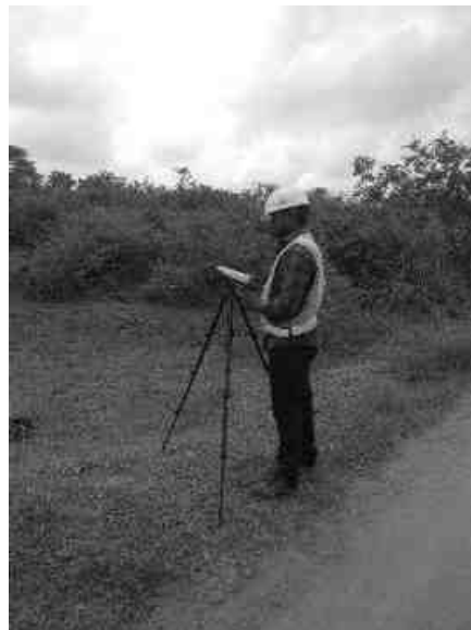
FIGURE 3.19. Collection of Noise Sample
