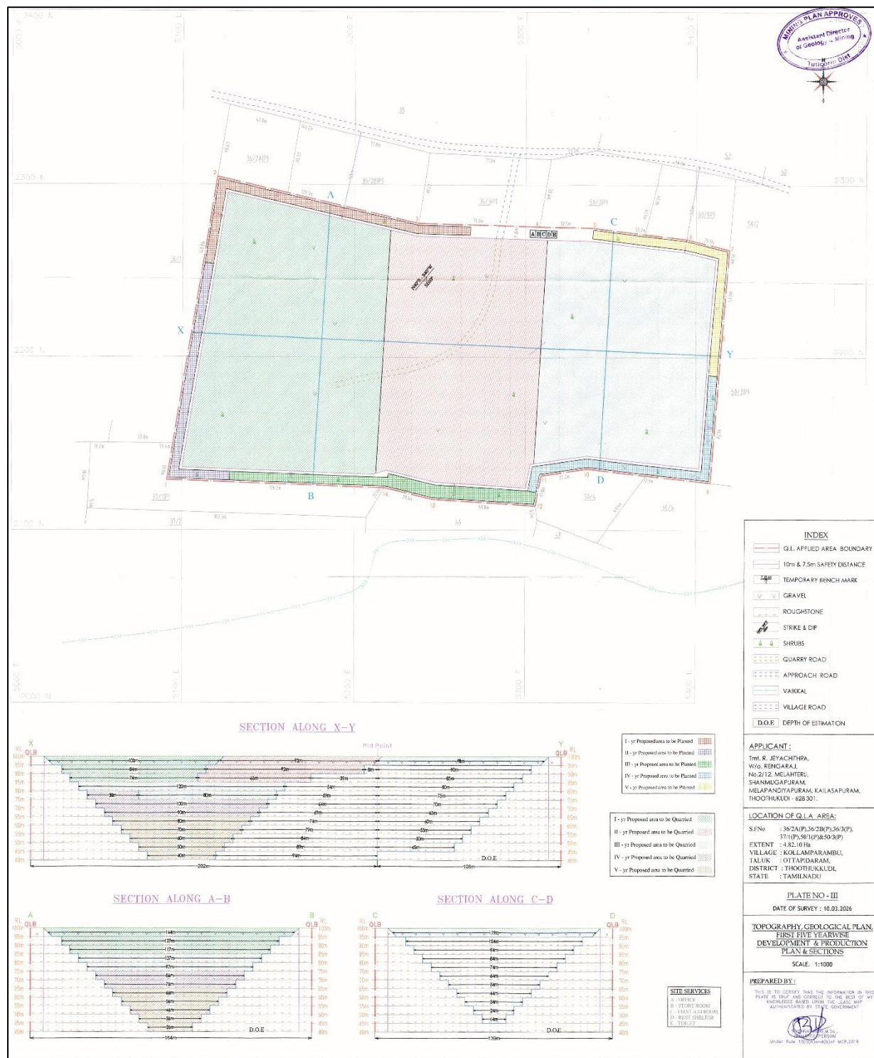
FIGURE 2.11: TOPOGRAPHY, GEOLOGICAL, YEARWISE DEVELOPMENT PRODUCTION PLAN AND SECTION FIRST FIVE YEARS
