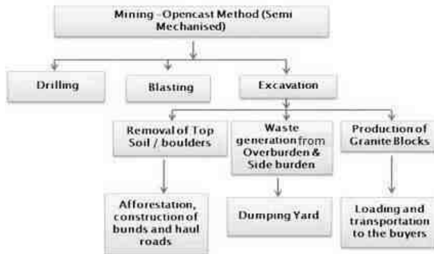
Figure 2-13 Schematic Diagram of Mining Process
