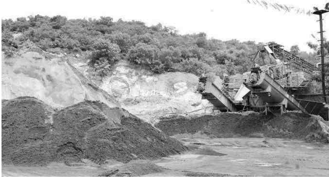
Photo: 28. Crushing Unit for preparation of M - Sand Manufactured Sand (M – Sand)
