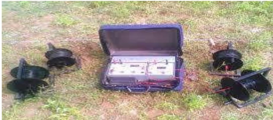
Fig. No. 3.23: DDR-3 Electrical Resistivity Meter
