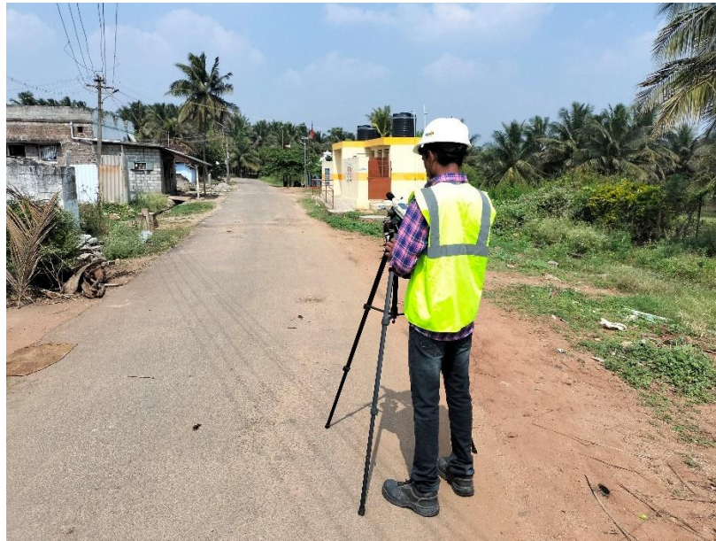
FIGURE 3.15: SITE PHOTOGRAPHS OF AMBIENT NOISE LEVEL MONITORING
