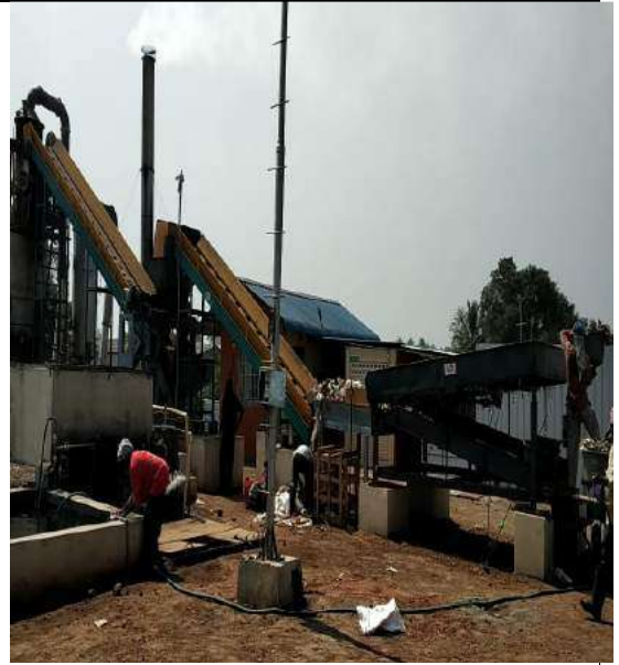
Green incinerator (50 T/day) at Vairapalayam MSW dump site which is under trial run
