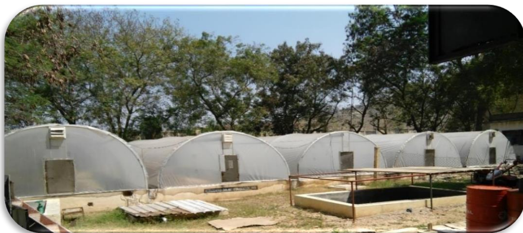
Reject Evaporation using Accelerated Solar Pan & Solar UV Tunnels
